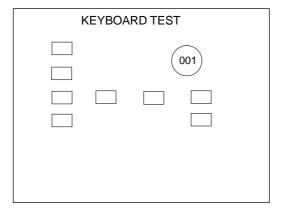
Operate each control on the control unit one by one. A key is functioning properly if its on-screen location lights in black when the key is pressed. For the [ENTER] knob, rotate it to show X-Y position; push it to confirm function.
